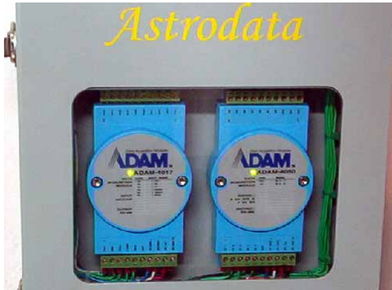
Figure 5-2: Two of the Astrodata interfaces, ADAM 4017 and ADAM 4050.
